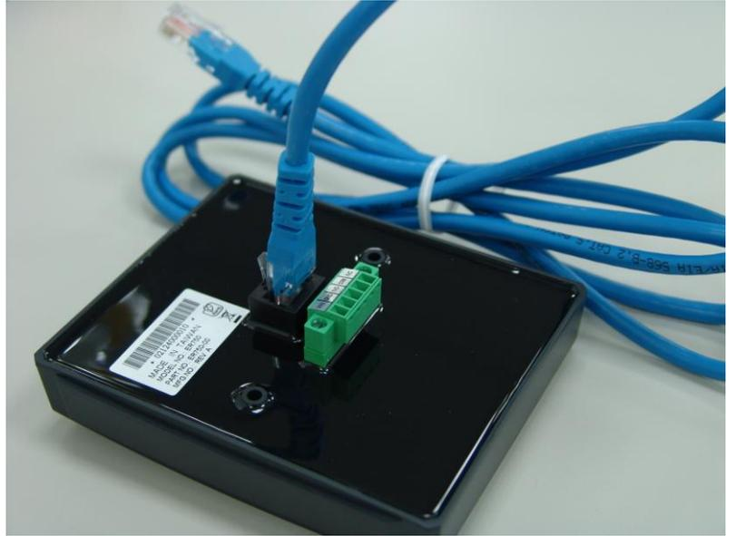
The ER750 does not supply power for the electronic lock, so please reference below pictures to connect the lock. Load means the lock. Connects VIN to power, GND to common, and the power supply's ground connect to NO (Normally Open).
