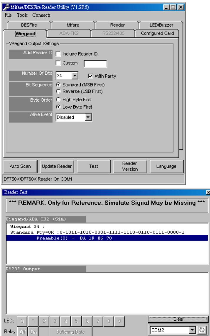
Remark: (1) When using reader-kit to test Wiegand (or TK2) signal, this test may be failed if the processor of computer is too slow. (2) When using reader-kit to test Wiegand (or TK2) signal, you need to connect to the physical COM port.
