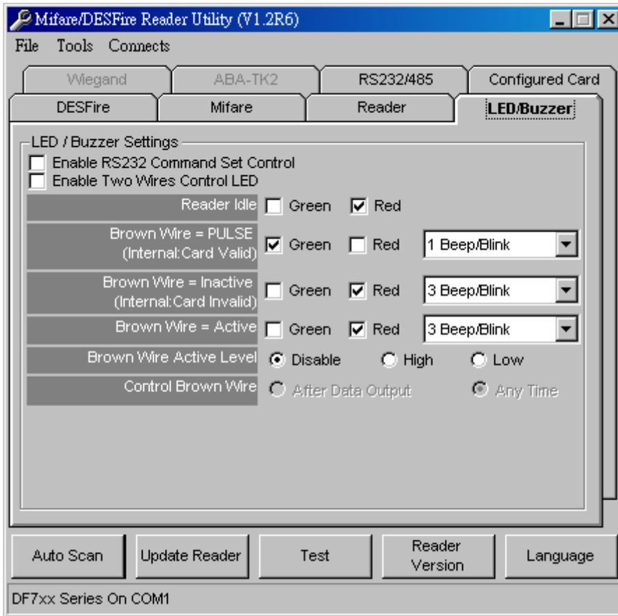
DF7XX supports LED/Alarm configure. Set the LED/Buzzer to indicate the system status for end-user.
