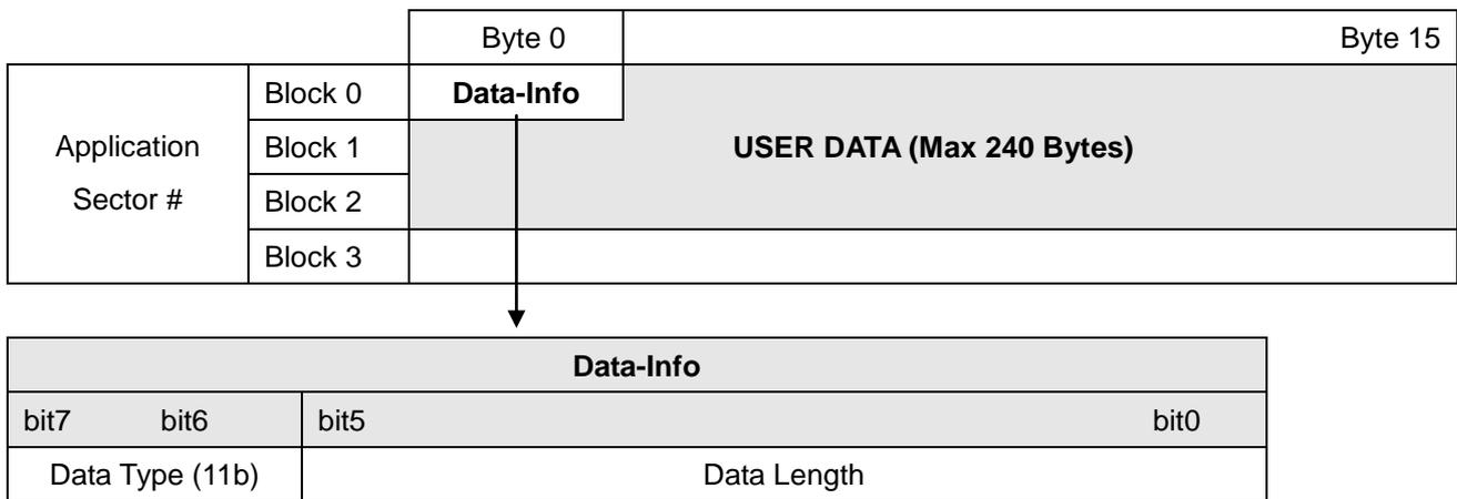
Data type is fixed with 11b which means "any other data" type of "Card Holder information" as MAD standard. And data length is including the data with ending zero "0", so the number of data byte sent by DF7XX is equal to data length with one less for RS232 output.
