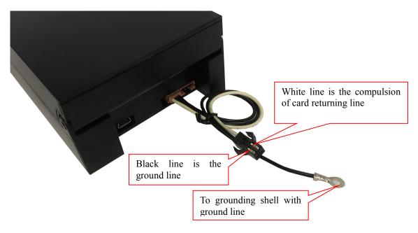
5.4 Backup power supply for ejecting card when power off ( achieve ejecting card when power off)
