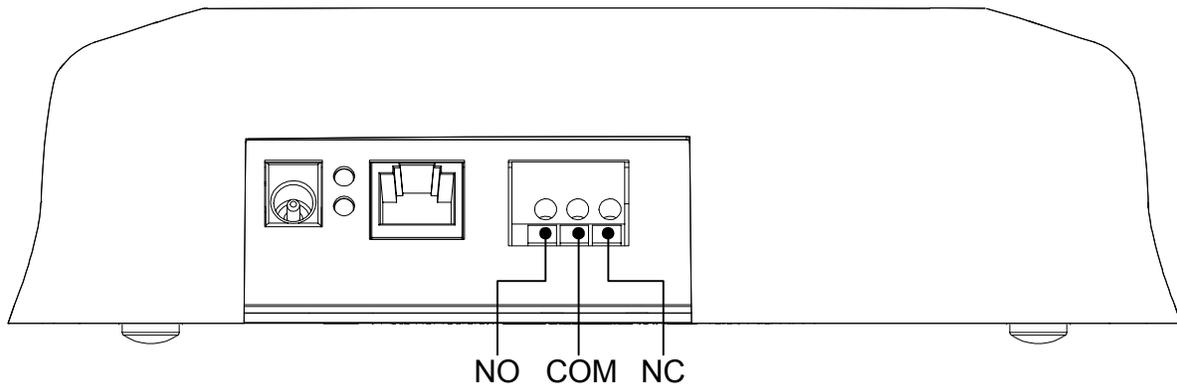
Relay connector is located under the metal back plate. Figure above shows connector position and pin assignment. Both Normally Closed (N.C.) and Normally Opened (N.O.) contacts are provided.
