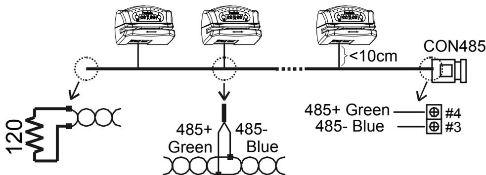
One side of the bus must be attached to the CON485: Blue connects to pin #3, Green connects to pin #4.
