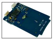
The ACM1281S-C7 Serial Contactless Reader Module with SAM Slot was designed based on the 13.56 MHz technology. It supports ISO 14443 Parts 1-4 Type A and B cards, and MIFARE® Classic series with a card reading distance of up to 50 mm (depending on tag type).
